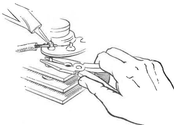
Fig. 20 Use of thermal shunt when soldering diode connections
