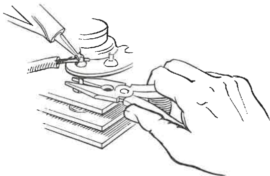
Fig. 13 Use of thermal shunt when soldering diode connexions
