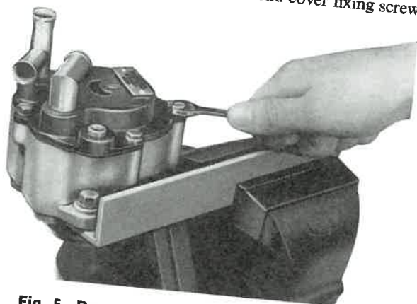
Fig. 5 Removing the port-end fixing screws
