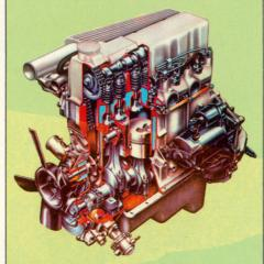
2 064cc (126 cu in) GM Diesel. Net power: 44 kW (60 bhp) at 4 400 rev/min.
