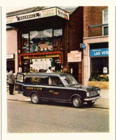
The heavy-duty HAV van combines all the features of the HAE van with heavier rear axle, springs and wheel equipment giving an additional payload allowance of 369 lb. (167 kg.) including driver.
