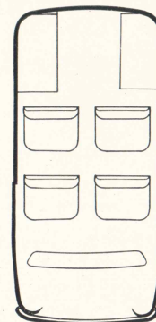
Rear seats folded down to form seating for two passengers each side
