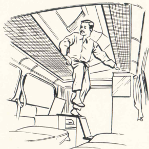
4-berth model. Access to upper berths by this folding step
