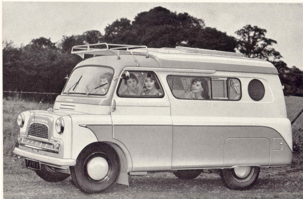
Here is the Bedford Dormobile Caravan (4-berth model) with the roof canopy folded down. The roof rack illustrated is an optional extra.
