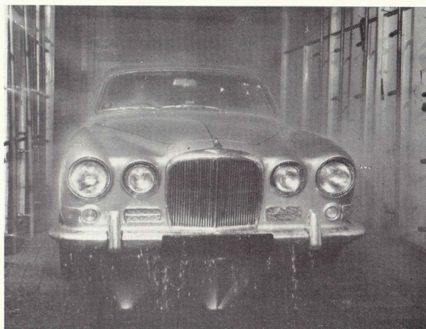
Completed cars are checked for water leaks in a special booth where nozzles direct water at the car from every direction.
