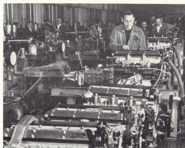
During the six hour run on a dynamometer in the test house each engine is subjected to a short power output/performance test, when fine adjustments are made to carburetters, ignition timing, etc.
