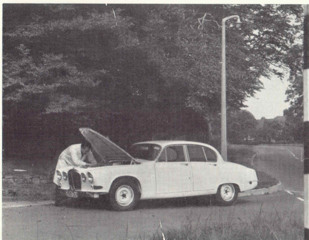
Every car is road tested on at least two occasions, each one by a different driver, who makes any fine tuning adjustments that are necessary.
