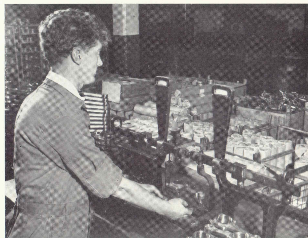
Connecting rods are checked for end to end balance with a tolerance of only 5 drams. Also centre to centre length is checked with a tolerance of 1/10,000 in.
