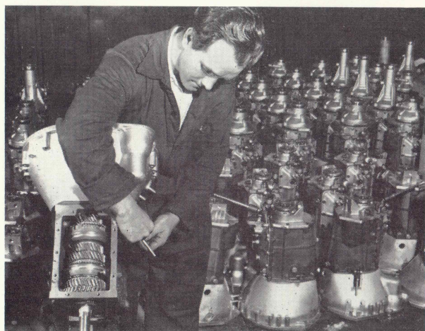
Selective assembly of gearbox components, followed by a test in a sound-proof booth, ensures that the unit is to a high standard.
