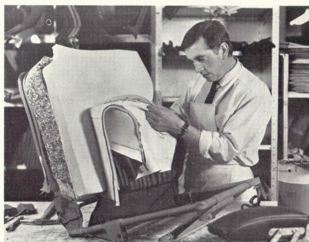
The trimming of cars is undertaken by highly skilled craftsmen who, to ensure uniformity within each car, select hides of matching grain and colour.
