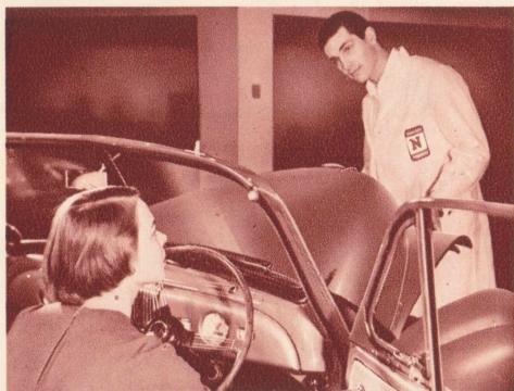
The bonnet catch is released from inside the car by gently pulling a control ring located under the instrument panel. As an additional precaution, the bonnet cannot be raised until the safety hook under the bonnet has also been released by hand. Morris one-piece bonnets are light and easy to handle—and allow maximum engine accessibility.
