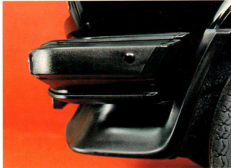
The front spoiler: increased tyre adhesion at high speed
