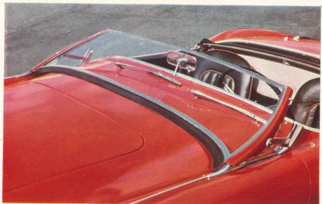
The windshield has two operative positions; raised, for normal driving conditions and lowered to form a scuttle when high speeds are anticipated. The change-over is readily effected and a positive locking device ensures absolute security in either position. The illustration (left) shows the windshield neatly lowered and enclosing such protrusions as windshield wipers and driving mirror.
