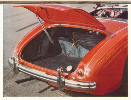
An exceptionally spacious luggage compartment for this type of car is provided at the rear. It also accommodates the spare wheel in a separate recessed shelf and encloses the fuel filler pipe.
