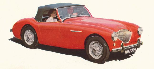
A specially tough fabric hood completes the comprehensive all-weather equipment of the Austin-Healey '100'. It folds away behind the seats when not in use, and can be quickly erected when necessary.
