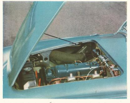
The bonnet top is hinged along its forward edge and opens widely to give good access to the engine and ancillary components for routine maintenance.
