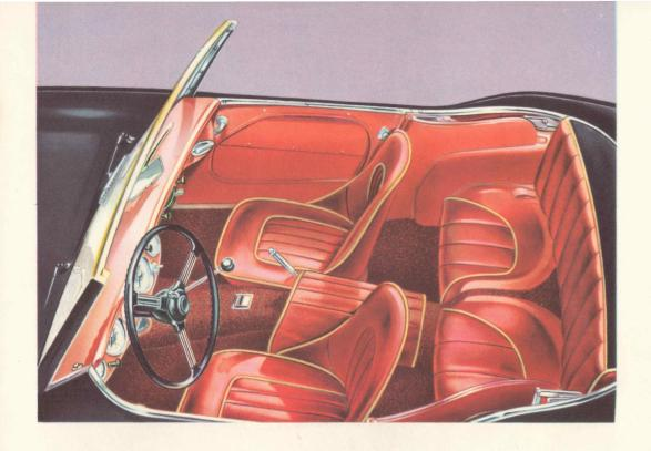
Each of the adjustable bucket seats in the neatly designed interior is upholstered in latex foam rubber, with hide facings. The backs tilt forward to give access to the rear seats.
