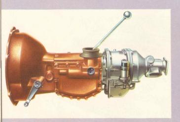
An electrically controlled overdrive (illustrated above) can, if required, be fitted to the standard four-speed synchromesh gearbox of the Austin Healey "100 Six." This is operated by a switch on the fascia and provides a high top gear ratio giving the car a fast cruising speed, while maintaining a modest fuel consumption. Whether steel disc or wire spoked knock-on wheels are used they must be equipped with Road Speed tyres when overdrive is fitted.
