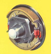
Large diameter hydraulic brakes with two-leading-shoe action on the front wheels ensure powerful and progressive retardation.
