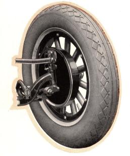
The new four-wheel brake mechanism is scaled from exposure and operates through steel cables
