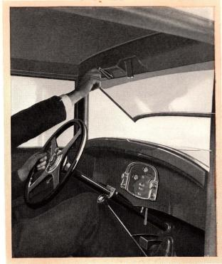
A crank type regulator within easy reach controls the windscreen in any position
