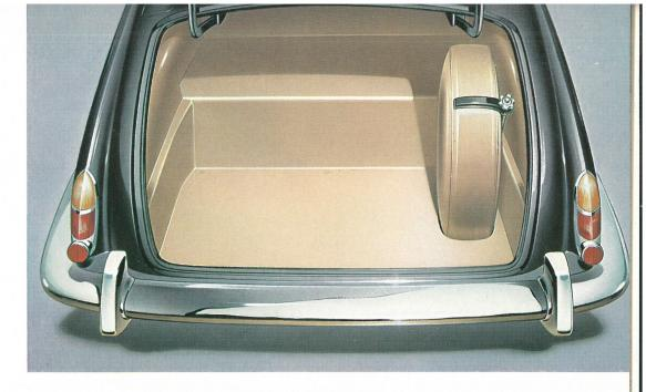
The luggage boot has a volume of 27 cubic feet excluding the space taken by the spare wheel and tool container. These are readily accessible without disturbing the luggage. The boot and spare wheel are fully trimmed in order to protect luggage.
