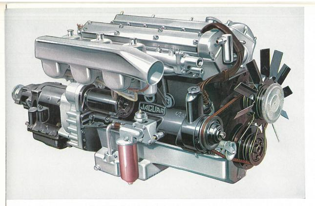
NEW ADVANCED XK ENGINE. 4.2 litre, 6 cylinder, twin overhead camshaft advanced design of race-proved, 3 carburetter, Jaguar XK engine, five times winner of Le Mans, gives higher torque for increased acceleration and flexibility.
