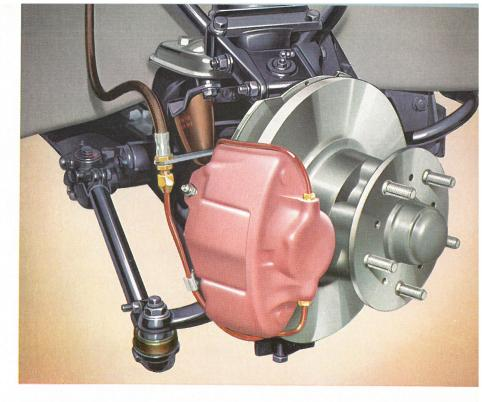
NEW EFFORTLESS BRAKING. New brake servo gives lower pedal effort and greater power for the disc brakes on all four wheels. Independent front and rear hydraulic systems provide important safety factor.
