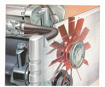
NEW ALTERNATOR. Alternator now gives greatly increased current supply over wide range of engine speeds, ensuring adequate current supply—even with city driving—for the extensive electrical service now embodied.
