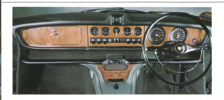
The modern facia, styled into the 420, features an extremely pleasing yet practical array of instruments and finger tip control switches set in a polished walnut panel which has a protective padded surround.
