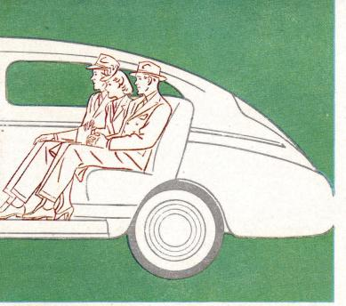
Note in the picture above how the low roof line does not afford ample head room. Nor do the shallow rear quarter windows provide generous vision. Compare with diagram at right.
