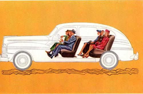
The new Mercury has mid-section seating. Rear seat passengers are located well ahead of the rear axle center line where the least amount of car movement occurs when negotiating rough roads. The result: a smoother, more level ride. Balanced weight distribution in combination with new slow-motion multileaf springs and a 129.38 inch spring base results in a full-cushioned ride.
