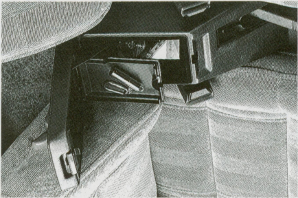
Centre Arm Rest Storage Box holds up to 7 cassette tapes, and has a "secret" space for credit cards and documents. (excl. GL)
