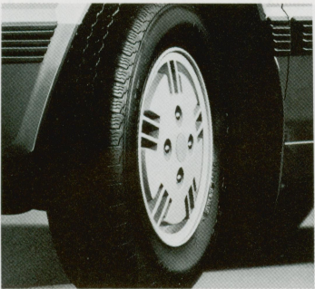
185/70 SR-13 SBR tyres with light alloy wheels
