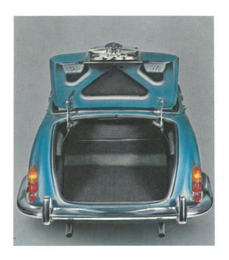
The wide and long boot of the Daimler Sovereign provides no less than 19 cubic feet usable capacity, which accommodates with ease the luggage of five people. It is fully trimmed throughout and is illuminated at night. Spare wheel and tools are carried in a separate compartment beneath the luggage boot floor.
