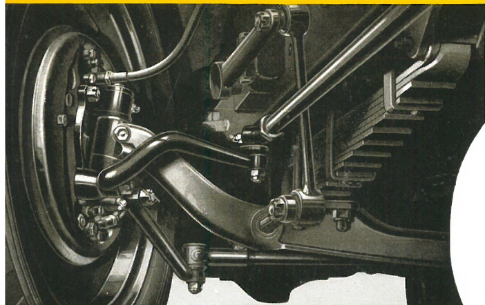
The front axle changes from I to rectangular section from the spring pads to the steering swivels giving great strength at a vital point while another feature of this assembly is the wide-lock steering.
