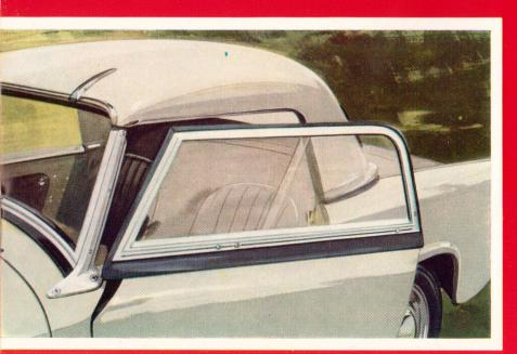
When not in use, the vinyl-treated fabric soft top and the metal frame can be stowed in the trunk. The quickly detachable, light-alloy frame side-screens have a sliding window which is easily adjustable for ventilation or hand-signaling.
