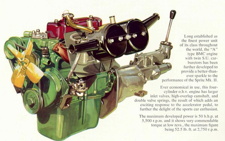
The four-speed, close-ratio gearbox has synchromesh engagement on second, third and top speeds. A scintillating "third gear" makes full use of the Sprite's acceleration and adds generally to its "grown-up" performance.
