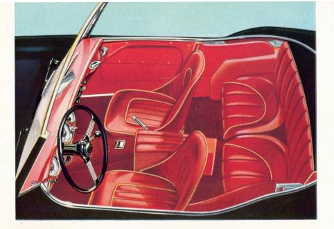
Each of the two front seats is adjustable. The seat cushions are removable and the squabs tilt forward to facilitate access to the inset well-type rear seats. An ash tray is provided in the centre transmission tunnel. On both two- and four-seater cars a master switch operates from inside the luggage compartment, which has a lockable lid, enabling the car to be safely left unattended.
