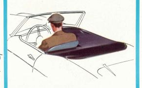
Included in the comprehensive all-weather equipment of the two- and four-seater Austin Healey "3000" Mk.II is a tough vinyl treated fabric hood which can be speedily erected or folded away as necessary. Also provided is a tonneau cover of similar material which can be opened for driver only, or for driver and passenger, until it can be completely removed and stowed away in its specially designed wallet.
