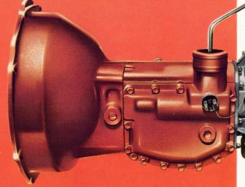
The basic two or four-seater Austin Healey "3000" Mk.11 is equipped with a four speed gearbox which has synchromesh engagement on second, third and top speeds. All components are subjected to rigid scrutiny and testing before assembly to ensure maximum efficiency in operation. Power is transmitted to the three quarter floating hypoid rear axle by an open propeller shaft with needle roller universal joints.
