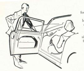
For ease of entry, forward hinged doors open wide and the lower edges lift well clear of the kerb or sidewalk.
