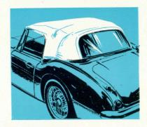
Truly, an all-weather car, the Sports Convertible has a tough, vinyl treated fabric hood which can be folded away behind the occasional rear seats in a matter of seconds—or just as quickly be re-erected! With hood raised, the interior takes on saloon-car comfort with friction controlled ventilating louvres and wind-
