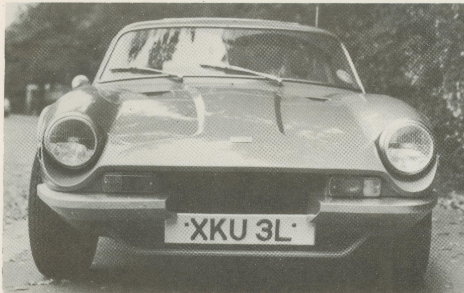
THE FRONTAL ASPECT of the latest TVR has been changed considerably in order to accept the spare-wheel forward of the radiator.
