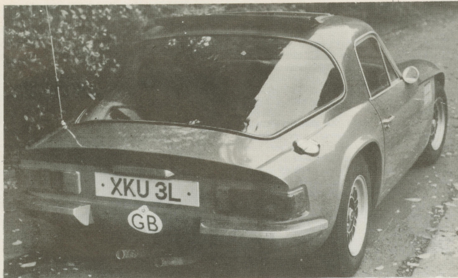
THE HEATED, panoramic rear screen gives good vision, though the quarter panels are awkward at road junctions. An impending new model will have a lift-up tail gate.
